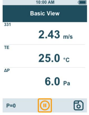
Depending on the connected probe, parameters can be configured for the measurement, for example, visibility of individual values or units.
