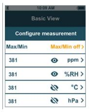
Individual values being hidden does not affect the application, only the Basic View and long-term measurement. The configured units, on the other hand, are also taken up in the application menus.
