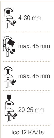
MPE Low voltage clamp
