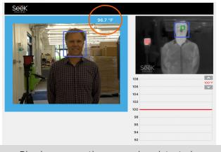
**4.** Blue box means the camera has detected a person and is measuring skin temperature.
