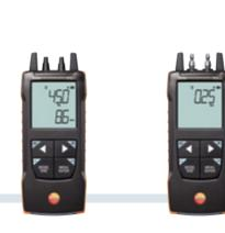
Differential pressure measuring instrument
