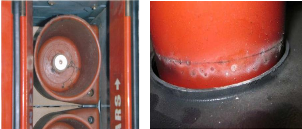
Figure 47 - Photos of surface tracking where black carbonisation (left) and white discoloration (right) can be seen.
